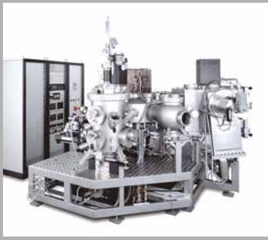
Cluster tool coating system for the production of X-ray mirrors.
