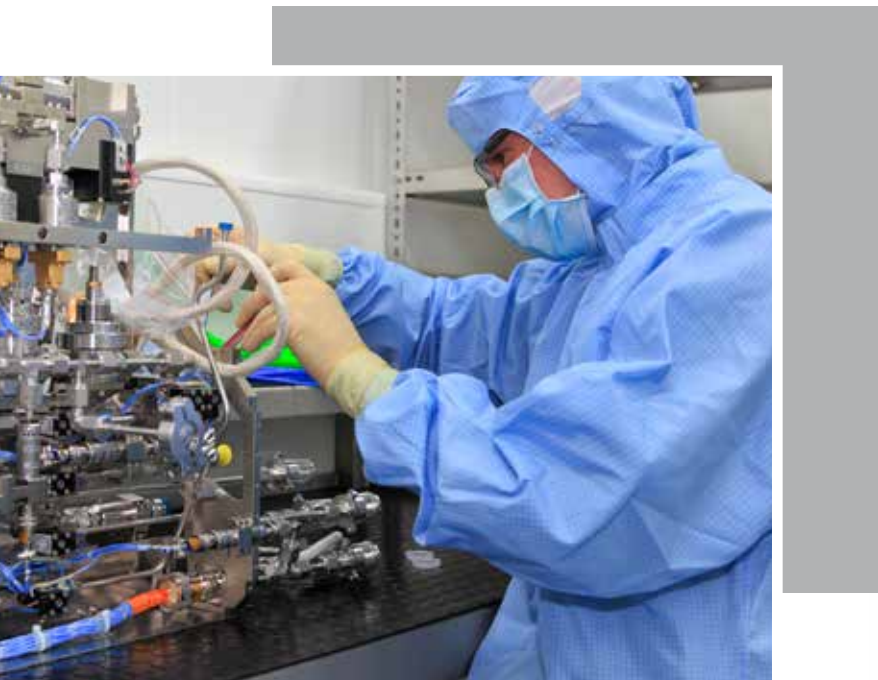
Cleanroom assembly work on the ultra-high vacuum chamber of the EML materials research module.
