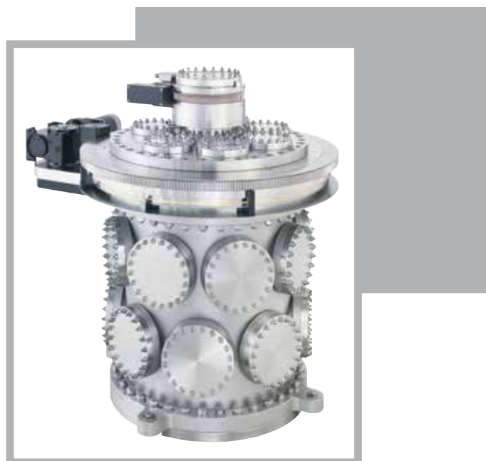
Vacuum measurement system for basic research (leak rate \leq 10^{-9} mbar x l/s), among other things with 2-fold differentially pumped DN 160 CF and DN 500 COF rotary joints and a position measurement system (angle accuracy 0.001^\circ ) powered by a stepping motor (rotary speed \sim 0.5 rpm).
