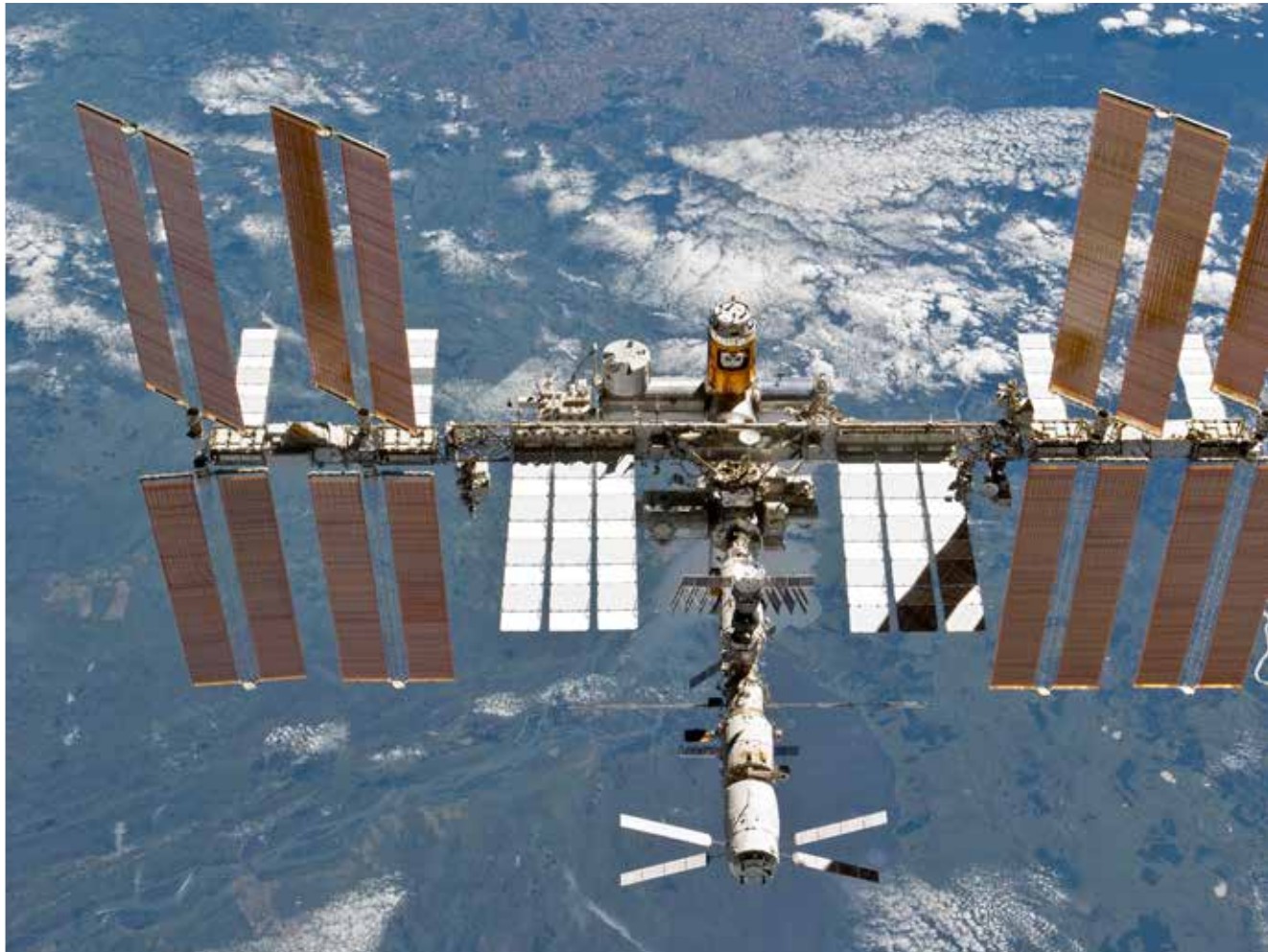
View from space of the International Space Station and the earth. On the right next to the central, gold-coloured module is the European space lab COLUMBUS. PINK is producing numerous systems for this, some of which are already installed. These also include about 400 running metres of ¼ " to 2" ducts and lines. Docking in the foreground is the ATV space transporter for which PINK has produced further components.
