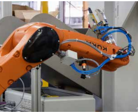
Design of a fully automatic helium leak test system with robots for the transfer of test specimens within various process stations.
