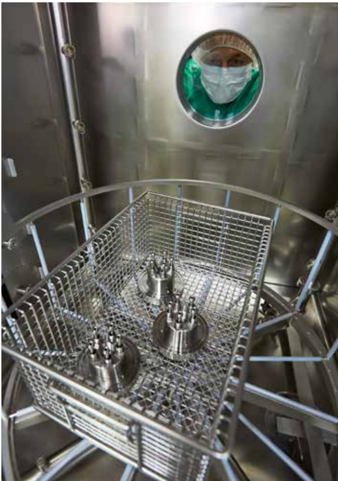
This vacuum cleaning and drying unit developed by PINK is designed for fully automatic operation.
